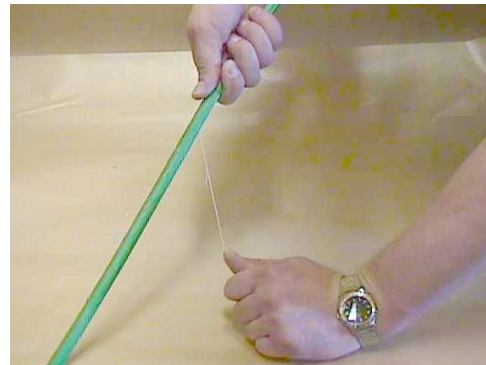
Stripping cable using the tear thread
