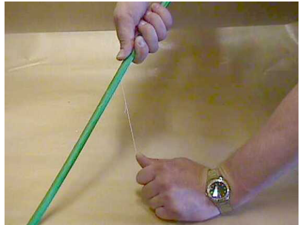
Stripping cable using tear thread
